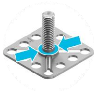
Shoulder diameter to suit ISO 273 clearance holes
