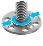
Shoulder diameter to suit ISO 273 clearance holes
